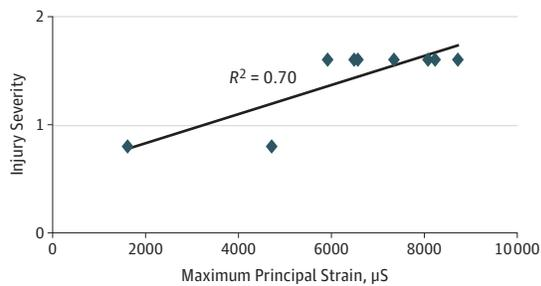
Each data point represents an orbital floor fracture.  $\mu\text{S}$  indicates microstrains.
