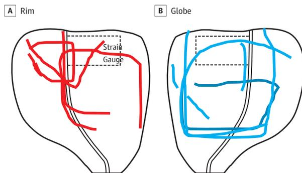
A, Rim; 3.86 J; maximum strain 5419 microstrains ( $\mu\text{S}$ ); minimum strain,  $-6906 \mu\text{S}$ ; maximum shear, 5395 Pa. B, Globe, 3.88 J; maximum strain, 6275  $\mu\text{S}$ ; minimum strain,  $-6043 \mu\text{S}$ ; maximum shear, 6085 Pa.
